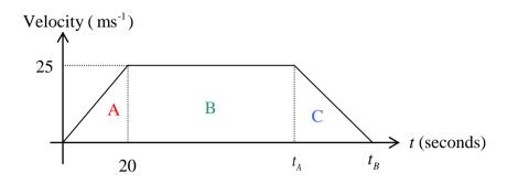
Area A + B + C = 2100 (area under graph = distance travelled) C = 125 (from question), A = 250 (using area of triangle), so: B = 2100 - 125 - 250 = 1725.
