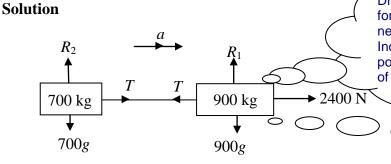
Draw a diagram and put on all forces, even those you may not need, e.g. reaction and weight. Include an acceleration arrow, pointing in the direction of motion of the system.
