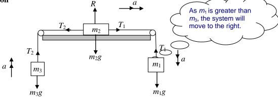
Mass  $m_1$  moves down, so the equation of motion for  $m_1$  is
