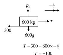
So the tension in the tow bar is 100 N and as it is negative it must be keeping the car and trailer apart, so the tow bar is in compression or thrust.
