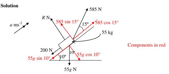
(i) Using Newton's second law parallel to the slope:
