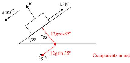
(i) Using Newton's second law perpendicular to the slope:
